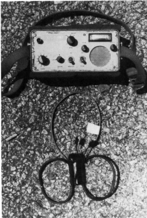
Figure 28. Portable 27 MHz radio receiver and radio transmitter used for instrumentation.
